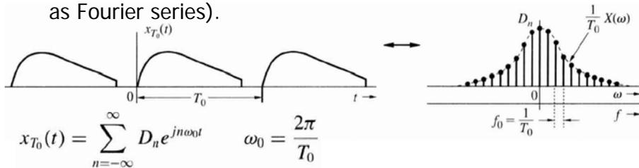
where  $D_n = \frac{1}{T_0} \int_0^{T_0} x(t) e^{-jn\omega_0 t} dt = \frac{1}{T_0} \int_0^{\tau} x(t) e^{-jn\omega_0 t} dt$
